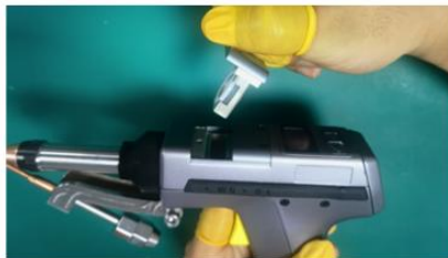
② Remove the protective lens holder
