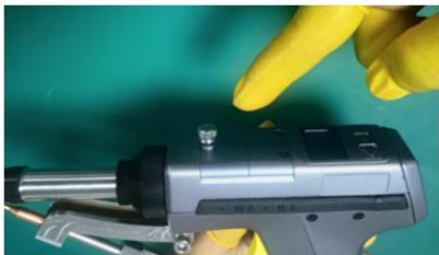
① Unscrew the protective lens screw
